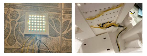
Cut two pieces of 22 gauge wire, one black, and one yellow to 24" (70cm) or so. Route them through the end hole of the LED Lightsource Box. Cut a strip of 6 LEDs (two strips) and solder the yellow to positive and the black to negative in the middle of the strip as shown below.
