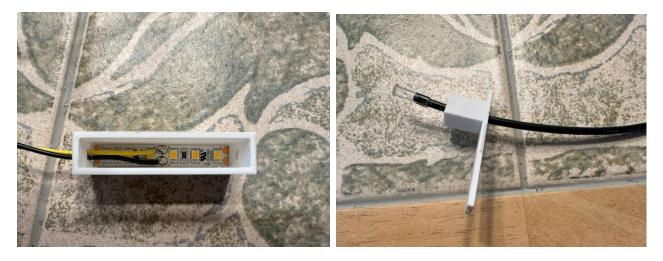
Snap the top to the bottom. You can test the lightpipe by putting 12V power to the LEDs. Glue the top to the bottom with some hot glue (not shown).
