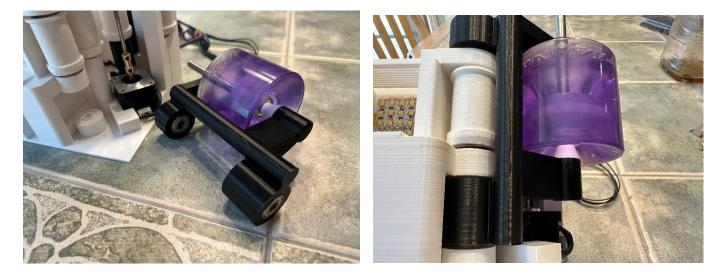
Hang two Small Swinging Arms with 8mm rods and bearings on the back wall. Put two properly sized flywheels (with bearings) on the arms. Put appropriately sized flywheels (with bearings) on all of the remaining spots.
