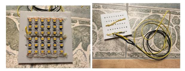
If you have a 12V power supply of some sort, test that the LEDs all light properly by hooking positive to Yellow and negative to Black. Install the panel in the Main Frame as shown and run the wires through the hole in the back. Hot glue the wires down as shown to keep them in the bottom of the unit and out of the way of where the tensioner arms will be swinging.
