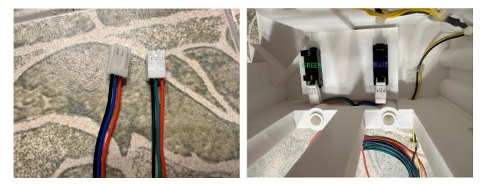
Hot Glue the sensors into Main Base on the bottom. Connect the two Red wires to a single Precrimped wire. Repeat for the two Black wires. Connect the Green and Blue wires to a pre-crimped wire each. You should now have four pre-crimped wires.
