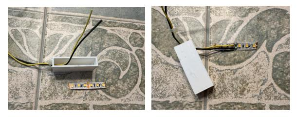
Peel the adhesive from the strip and put it at the bottom of the box. Put the Lightpipe through the box top as shown.
