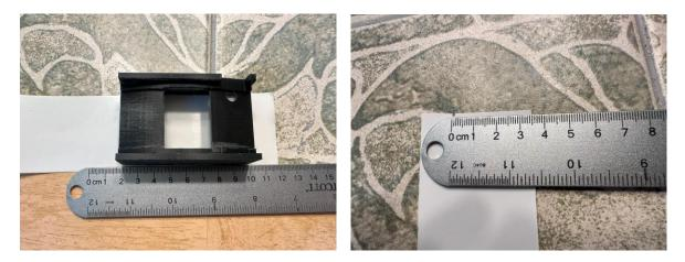
Cut the strip along the line with a razor or scissors. Note, keep the remaining tape, you can use it on a 16mm or smaller gate in the future. The tape should fit inside the track on the gate.
