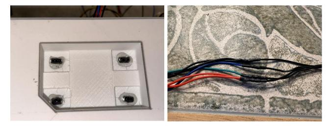
Connect the Black Wires on the Left, The Red Wire next to it, followed by Blue and then by Green. Mark this cable to distinguish it as the sensors. If this is accidentally plugged into one of the motor connectors on the PCB, it will destroy the sensors.
