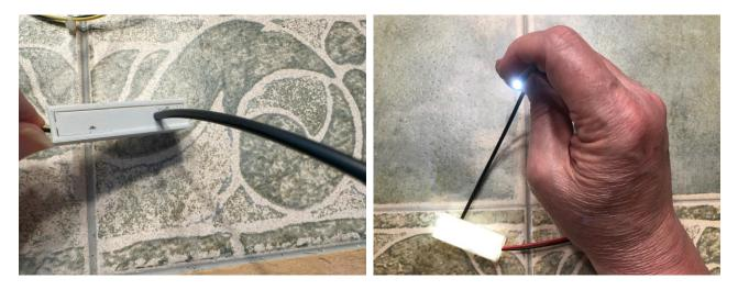
Cut the Yellow and Black wires coming out of the back of the unit to about the 4" (10cm) point and strip the wires. Connect the LED Lightpipe wires to LED Back Panel with the remaining wires you cut off by twisting, hooking, soldering and covering with heat shrink tubing. You now have a single set of wires to power all of the LEDs.
