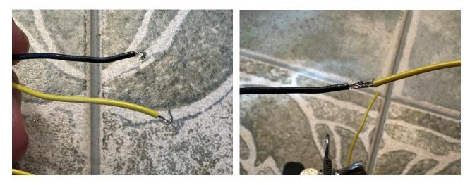
Solder the wires together. Cover with shrink tubing and use a heat gun to shrink the tubing. Remember that you might need to put the shrink tubing on prior to making the connection.
