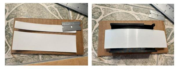
Cut the strip in half, peel, and wrap it around the left side of the gate. Trim so it doesn't overlap on the back.
