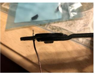
Push the pins into the Connector Housing. Use wire ties to hold the wires together for the length of the wires.
