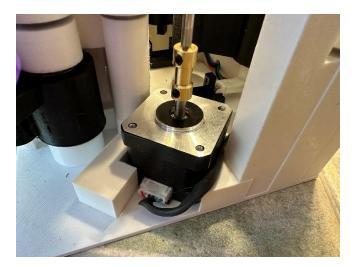
The motor has two windings internally and the datasheet for your motor should show you what two wires go to each winding. In our case, the [Green and Red] and the [Blue and Yellow] are how they are assigned. Connect all 4 wires from the motor to 4 separate pre- crimped wires. Connect the proper pairs into a connector keeping them together. It doesn't matter which pair is on either side as long as they stay together.
