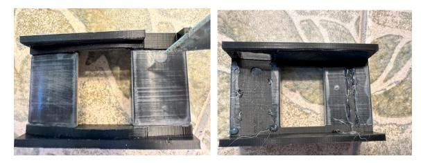
Test that the hole detector fits all the way on the gate. The Gate is completed. Repeat for any other formats you plan to scan.
