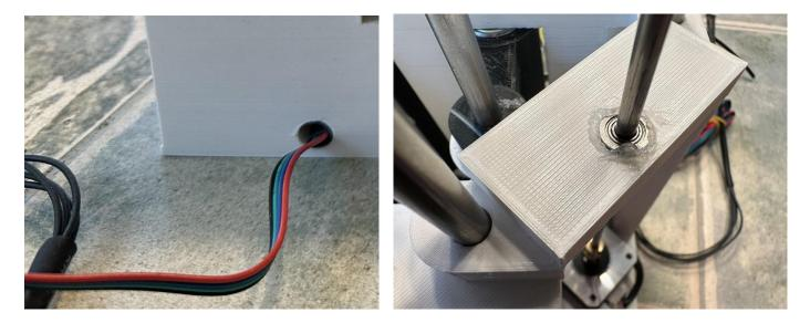
Put the motor in the base with the cables routed behind it. Attach the 4mm to 5mm Brass Shaft Coupling Joint Connector with the 5mm side clamped onto the motor. Push the 4mm Rod through the bearing at the top and clamp it to the motor at the coupling joint.
