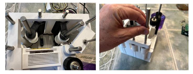
Cut the Matte Archival Polyester Film into eight squares that are 65 X 70mm each. There is a template available on the Wiki page to print the cutting lines with a laser printer on the film. Insert the Theatre Sleve in the front of the theatre. Secure it by inserting filters through the top of the Theatre.
