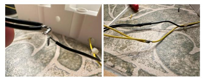
Attach the Yellow wire to a Pre-Crimped wire. Do the same for the Black wire and cover with shrink tubing. Push the ends of the pre-crimped wires into a Housings Receptacle with the Yellow wire on the right and the Black wire next to it as shown below. Use wire ties to hold the wires together for the length of the wires.
