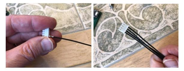
Use Wire Ties to keep the wires together. Warning: Resist the urge to twist or braid the wires together. This can cause interference issues.
