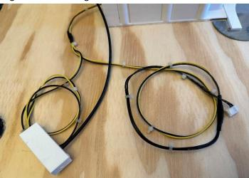
Test fit the Photocell into the Opto Coupler Bottom and cut back the leads a few millimeters so that wires will be insulated inside the coupler (older coupler shown in first illustration). Solder two 24" (70cm) 22 Guage wires of the same color to the ends of the leads.
