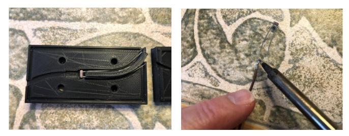
Position the Photocell in the Opto Coupler Bottom. Insert a Light Pipe as shown. Attach the Opto Coupler Top, and tape or Hot Glue the two halves together. Crimp a Connector Pin (WM2512-ND) onto each of the other ends of the wires.
