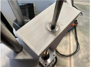
Put the motor in the base with the cables routed behind it. Attach the 4mm to 5mm Brass Shaft Coupling Joint Connector with the 5mm side clamped onto the motor. Push the 4mm Rod through the bearing at the top and clamp it to the motor at the coupling joint.
