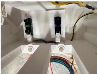
Hot Glue the sensors into Main Base on the bottom. Connect the two Red wires to a single Precrimped wire. Repeat for the two Black wires. Connect the Green and Blue wires to a pre-crimped wire each. You should now have four pre-crimped wires.
