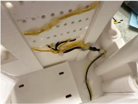
Attach the Yellow wire to a Pre-Crimped wire. Do the same for the Black wire and cover with shrink tubing. Push the ends of the pre-crimped wires into a Housings Receptacle with the Yellow wire on the right and the Black wire next to it as shown below. Use wire ties to hold the wires together for the length of the wires.
