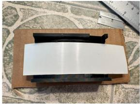
Cut the strip in half, peel, and wrap it around the left side of the gate. Trim so it doesn't overlap on the back.
