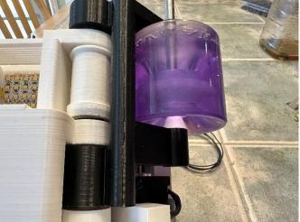
Hang two Small Swinging Arms with 8mm x 15cm rods and bearings on the back wall. Put two properly sized flywheels (with bearings) on the arms. Put appropriately sized flywheels (with bearings) on all of the remaining spots.
