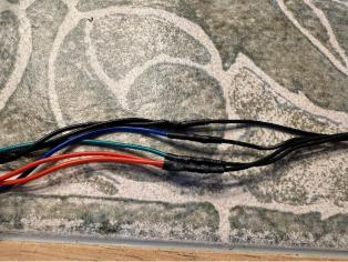
Connect the Black Wires on the Left, The Red Wire next to it, followed by Blue and then by Green. Mark this cable to distinguish it as the sensors. If this is accidentally plugged into one of the motor connectors on the PCB, it will destroy the sensors.
