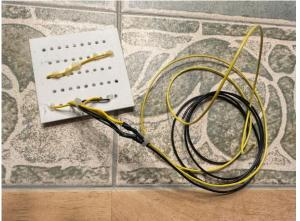
If you have a 12V power supply of some sort, test that the LEDs all light properly by hooking positive to Yellow and negative to Black. Install the panel in the Main Frame as shown and run the wires through the hole in the back. Hot glue the wires down as shown to keep them in the bottom of the unit and out of the way of where the tensioner arms will be swinging.
