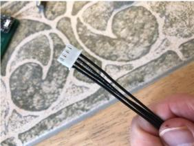
Use Wire Ties to keep the wires together. Warning: Resist the urge to twist or braid the wires together. This can cause interference issues.
