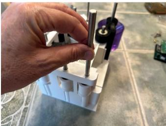
Cut the Matte Archival Polyester Film into eight squares that are 65 X 70mm each. There is a template available on the Wiki page to print the cutting lines with a laser printer on the film. Insert the Theatre Sleve in the front of the theatre. Secure it by inserting filters through the top of the Theatre.
