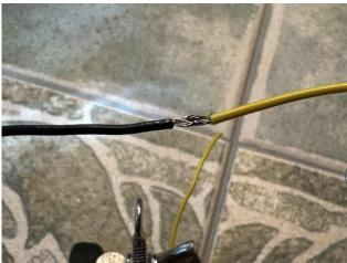
Solder the wires together. Cover with shrink tubing and use a heat gun to shrink the tubing. Remember that you might need to put the shrink tubing on prior to making the connection.
