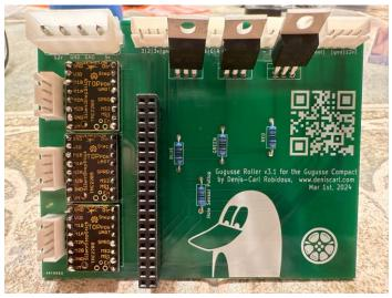
Install three Heatsinks on the motor boards and the PCB is complete.
