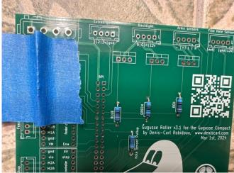
**Solder only one pin** on each of the rows of pins. Do this for both sides of the motor board. Test fit the motor board on the pins and if it doesn't fit, adjust the pins by heating up the pins and moving them until the board goes on. Solder all of the contacts on both sides of the PCB and repeat for the remaining two motor boards.
