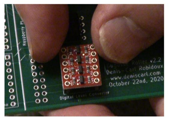
Repeat the process for the Arduino and the three Stepper Driver modules being sure that they are all oriented properly.
