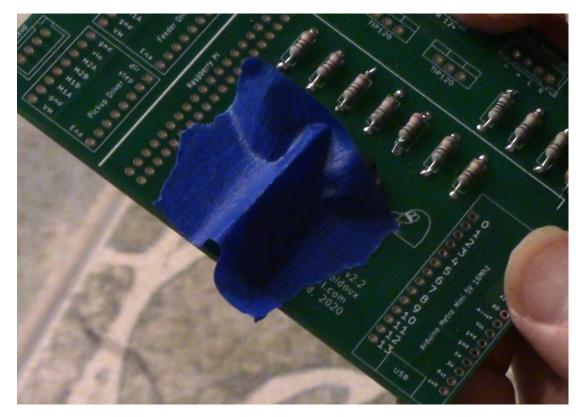
Solder only one pin on each of the rows of pins.
