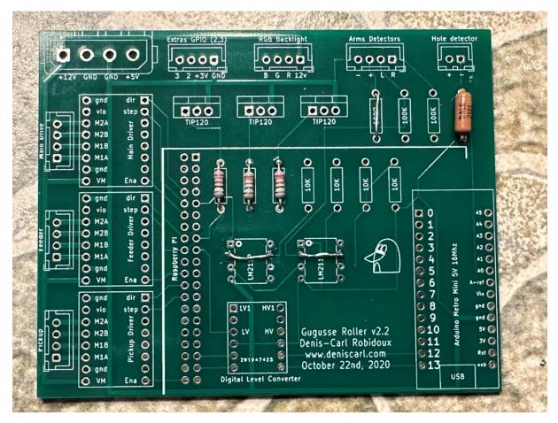
Insert 6 Support Pins for the Digital Level Converter with the long side going through the board.
