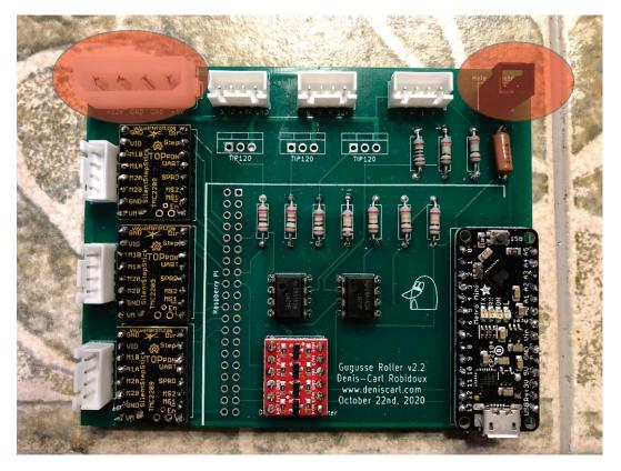
Follow this with the TIP 120 transistors and the 40 pin Raspberry Pi connector. Put some small heat sinks on the Stepper Driver controllers to dissipate some of the heat. Your board is complete.
