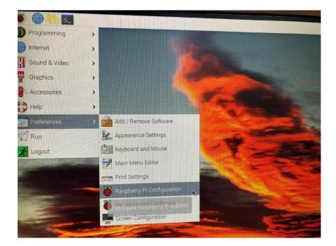
Click on the top Display Tab and set "Screen Blanking" to "Off". Click on the Performance Tab and set "GPU Memory" to 256 and click [OK]. Reboot when prompted.
