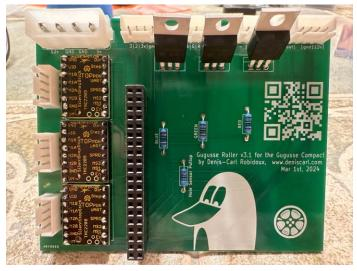
Install three Heatsinks on the motor boards and the PCB is complete.
