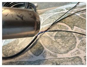
Put a piece of thick shrink tubing over all of the wires but before you shrink it, mark each of the ends with the colors or what they do based on the specs written on the side of the EX-DN10. Cover all 3 with a wider piece of shrink tubing. Match them up to the proper pins on the housing following the pinouts on the PCB or use the picture below.
